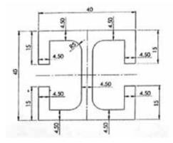
\* Special profile is designed for fixing solar panels with bolts.
