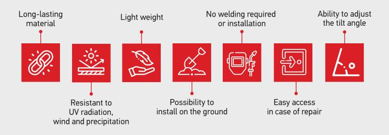
Fiberglass composite structures are ideal for aggressive environments as they are not subject to corrosion or electro-corrosion risks. That is why they are gaining more and more popularity in railway, port or urban infrastructure objects, as they are able to maintain their mechanical, functional and aesthetic properties for many years.
